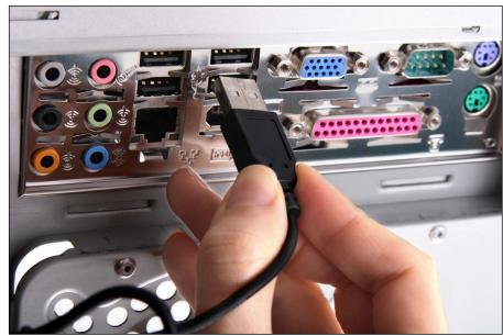
Figure 2-6: The ports on the back of a typical desktop computer.
