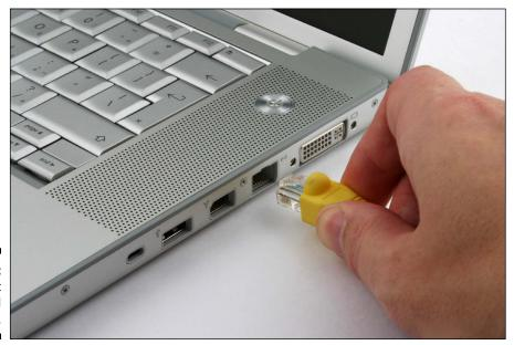
Figure 1-6: An Ethernet port and cable.
