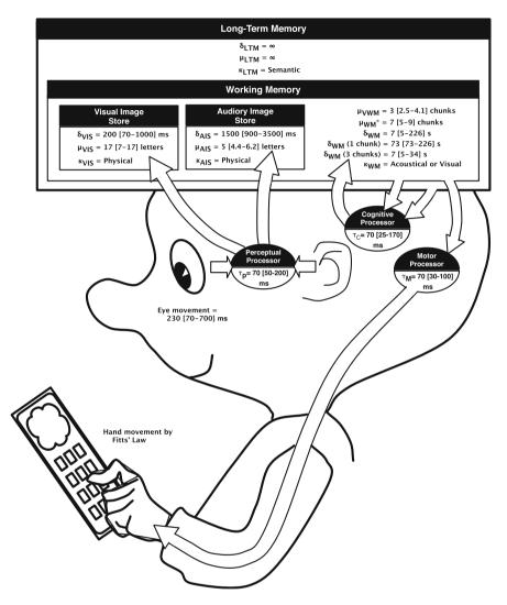
Fig. 14.2 A diagram of the model human processor (adapted from Card et al. 1983).  $\delta$  indicates a half-life decay rate;  $\mu$  is a capacity;  $\kappa$  is the modality of the storage;  $\tau$  is the time to do something
