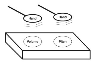
**Fig. 7.1** A diagram of a Theremin. Users play it by moving one hand closer to or farther away from the volume control and the other hand closer to or farther away from the pitch control. The distance is measured through capacitance. There are no fixed volumes or pitches, unlike most other instruments. It is sometimes used to make eerie sounds in science fiction movies
