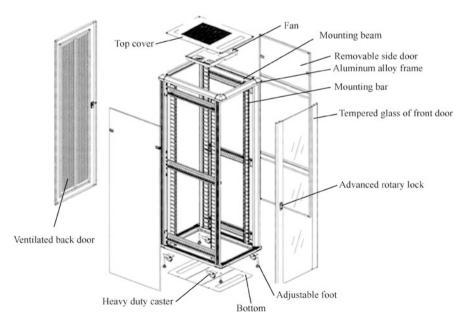
Fig. 2.2 Basic structure of network cabinet
