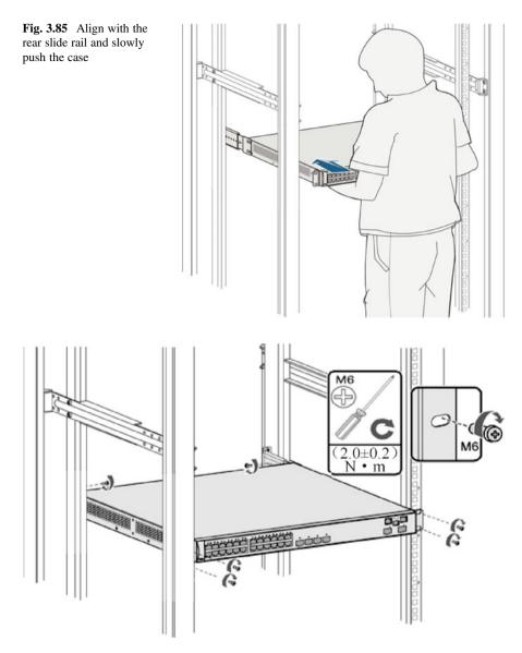
Fig. 3.86 Fix the rear mounting ears to the rear slide rail
