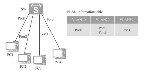
Fig. 4.20 VLAN allocation based on port
