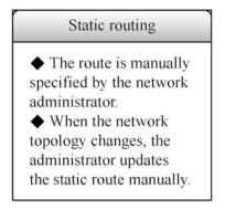
Fig. 4.30 Static vs. dynamic routing
