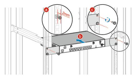
Fig. 3.31 Install the router into the cabinet
