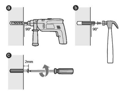
Fig. 3.27 Drill holes and mount the screws
