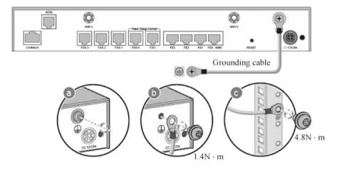
Fig. 3.32 Connect the grounding cable
