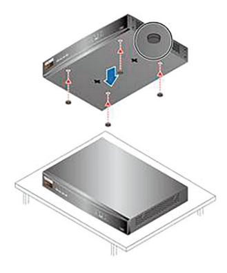
After the installation is completed, the following checks should be made: the USG device is firmly placed in the cabinet; there are no objects around the USG that hinder the heat dissipation.
