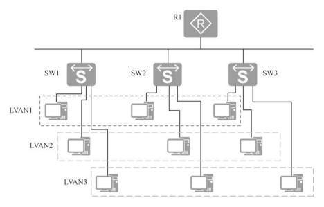
Fig. 4.17 Typical application of a VLAN
