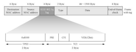
Fig. 4.19 IEEE 802.1q-based Ethernet frame format
