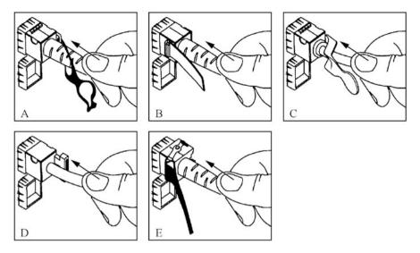
Fig. 3.80 Connect the high-speed cable to the switch interface
