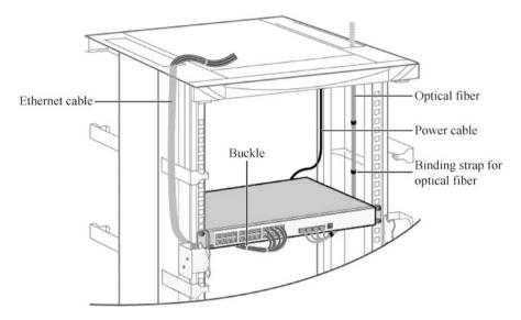
Fig. 3.90 When the cable connection is completed
