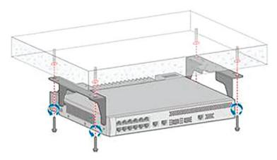
Fig. 3.70 Mount the switch to the ceiling
