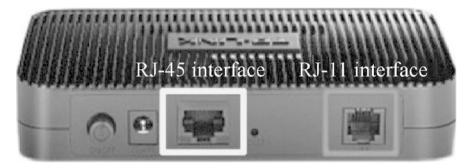
Fig. 2.36 Appearance of the two types of interfaces
