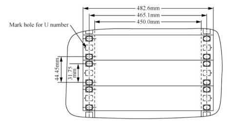
Fig. 2.4 The mounting dimensions of the 19-inch rack
