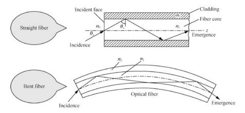
Fig. 2.26 Principle of optical fiber transmission
