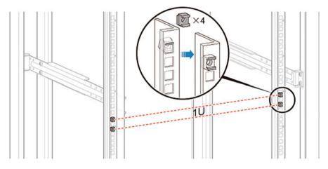
Fig. 3.30 Install the floating nuts
