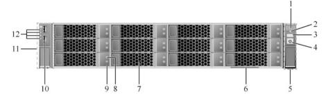
Fig. 3.22 Front panel of the RH2288H V3 (with 12 inch  $\times$  3.5 inch [approximately 30 cm  $\times$  9 cm] hard disks)
