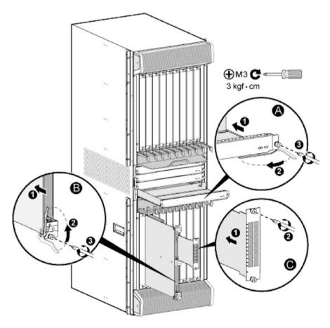
Fig. 3.52 Install the board and sub-board
