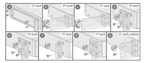
Fig. 3.60 Installation methods for different mounting ears
