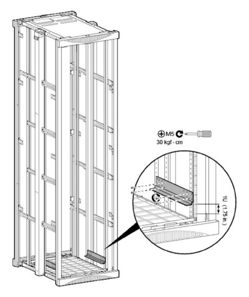
Fig. 3.38 Install the cabinet slide rails
