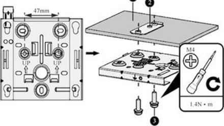
Fig. 3.97 Mark positioning points and drill holes. (1) Ceiling; (2) Clamping piece; (3) M4  $\times$  30 screw
