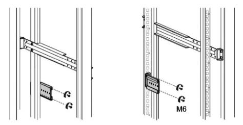
Fig. 3.84 Fix the slide rail for the rear mounting ears
