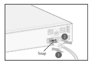
If the optical fiber needs to be removed, gently push the optical fiber connector inward, and then pinch the snap to pull it out, as shown in Fig. 3.79. It is prohibited to pull out the optical fiber connector directly. In the case that the interfaces are densely deployed and inconvenient to be operated by hand, the fiber extraction tool can be used to assist the operation.
