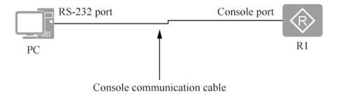
Fig. 5.5 Log in through the Console port
