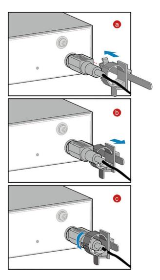
Fig. 3.35 Connect the power cable buckle
