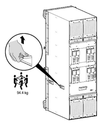
Fig. 3.37 Chassis handling method
