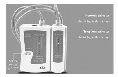
Fig. 2.50 Appearance of the Nengshou Network Tester
