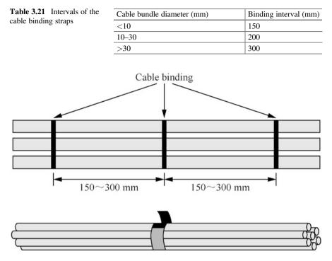
Fig. 3.77 Cable binding method
