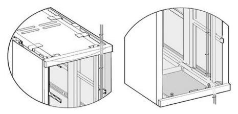
Fig. 3.122 Cabling between the cabinet (lower cabling [left] and upper cabling [right])
