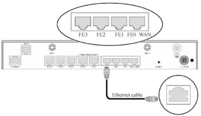
Ethernet port of the corresponding device
