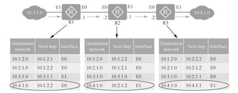
Fig. 4.26 Process of IP routing
