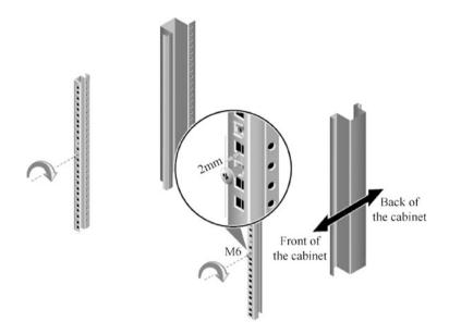
Fig. 3.106 Install the M6 screw into the cabinet
