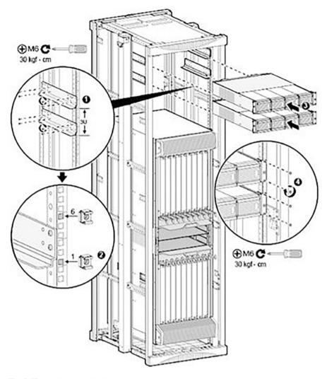
Fig. 3.45 Install the AC distribution box
