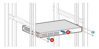
Fig. 3.64 Install the switch into the cabinet
