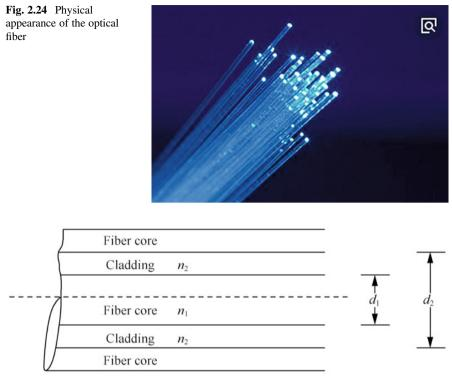
Fig. 2.25 Basic structure of the optical fiber
