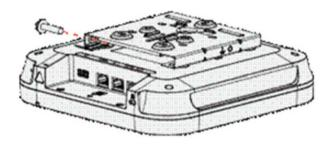
between the clamping piece and the sheet mounting lock, and finally lock the screws on the clamping piece, as shown in Fig. 3.100.
