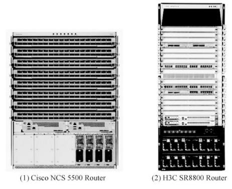
Fig. 3.2 Chassis-shaped routers
