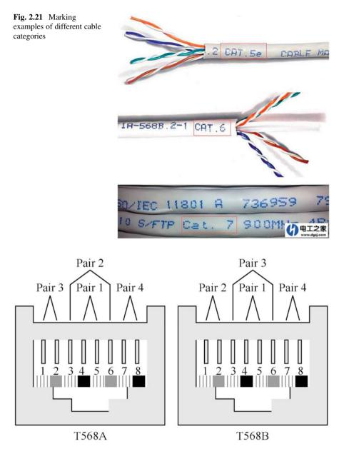
Fig. 2.22 Color labels and wire sequence of the TP
