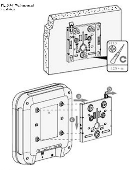
Fig. 3.95 Fix the AP to the wall
