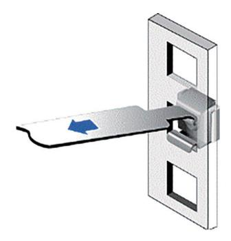
(i) Install the floating nuts, as shown in Fig. 3.115.
