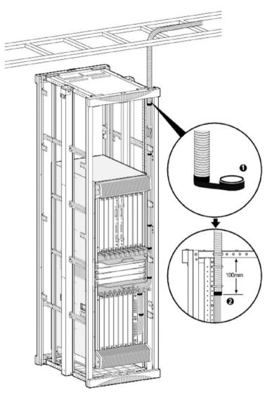
Fig. 3.56 Install the corrugated pipe
