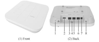
Fig. 3.16 Huawei AP7050DE Wireless AP
