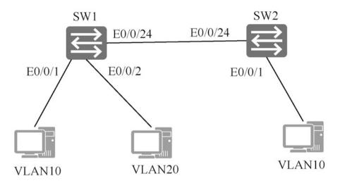
Fig. 5.23 Topology of VLAN's basic configuration
