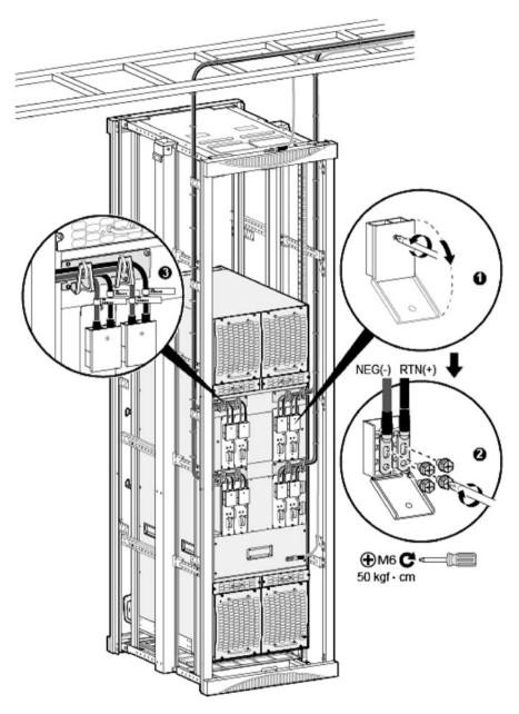
Fig. 3.42 Connect the grounding cable and PGND cable
