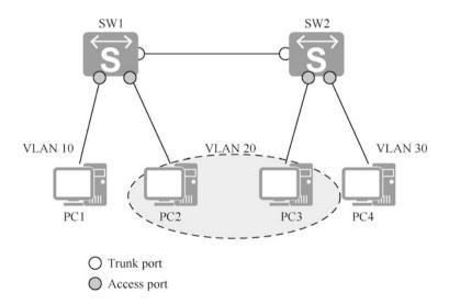
Fig. 4.22 Three different VLAN port types
