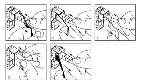
Fig. 3.81 Pull out the high-speed cable
