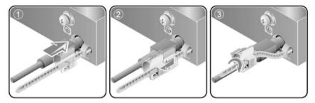
Fig. 3.112 Connect the power adapter
