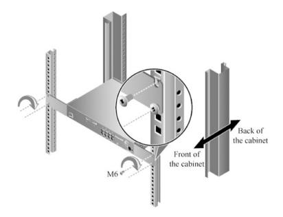
Fig. 3.107 Install the device into the cabinet
