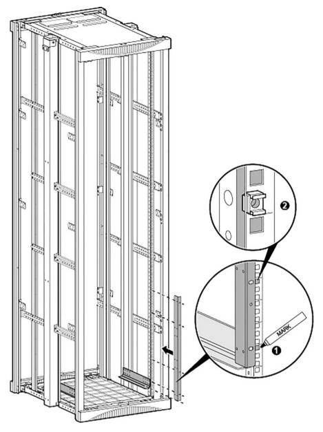
Fig. 3.40 Install the floating nuts
