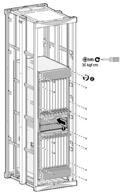
Fig. 3.41 Install the chassis in the cabinet
