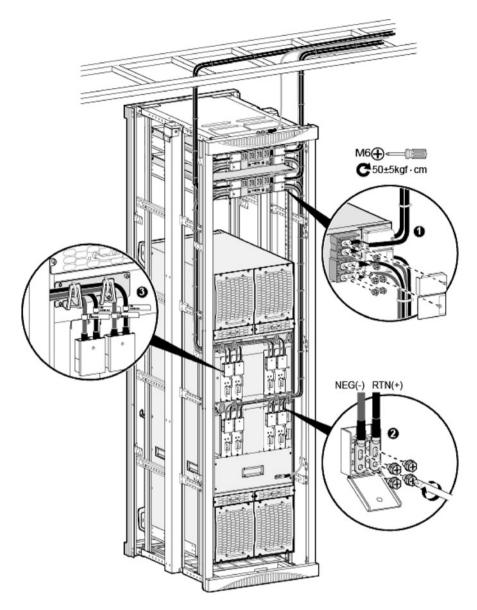
Fig. 3.49 Install the AC power cable
