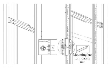
Fig. 3.83 Install the floating nuts
