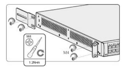
Fig. 3.82 Fix the front and rear mounting ears
