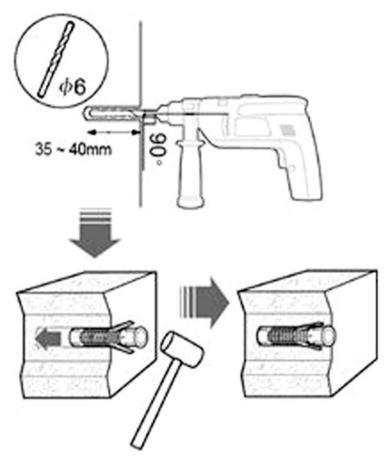
Fig. 3.93 Drill holes at the installation positions
