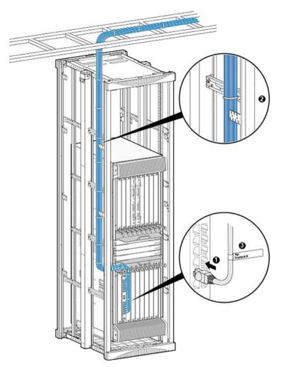
Fig. 3.53 Connect the network cable
