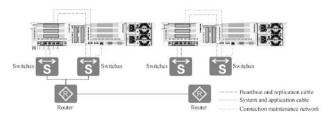
Fig. 3.120 Network cable connection of remote high-availability system
