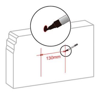
personal injury. Tools and accessories to be prepared include percussion drill, claw hammer, plastic expansion tubes and screws.
