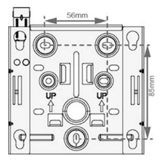
**Fig. 3.92** Mark the installation positions
