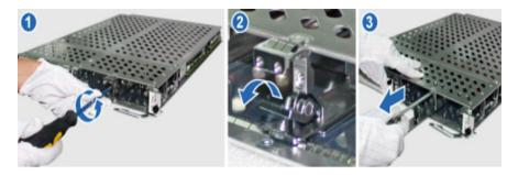
Fig. 3.51 Remove the redundant slide rails for sub-cards
