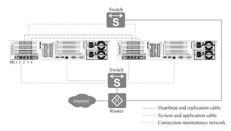
Fig. 3.119 Network cable connection of local high-availability system
