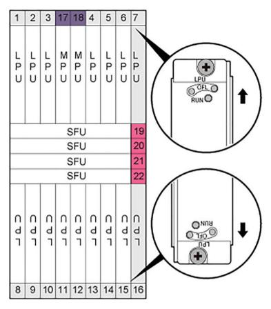
Fig. 3.50 Board slot layout
