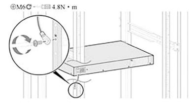
Fig. 3.63 Connect the grounding cable to the cabinet grounding point
