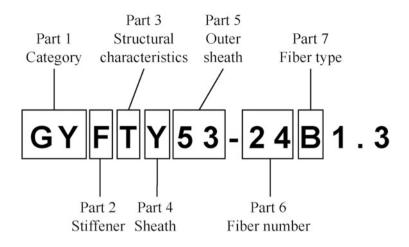
Fig. 2.33 Model of optical fiber cables
