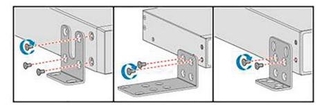
Fig. 3.67 Installation methods for different mounting ears
