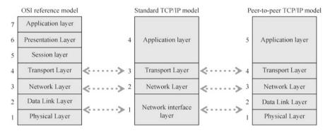
Fig. 4.5 The correspondence between the TCP/IP protocol cluster and the OSI Reference Model
