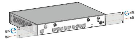
Fig. 3.29 Attach the mounting ears
