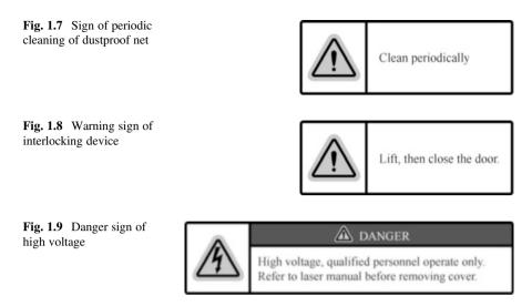
to be lifted by three people; Fig. 1.6 (3) indicates that the part or equipment weighs more than 55 kg and needs to be moved by a forklift or by four people.(c) Sign of regular cleaning of dustproof net
