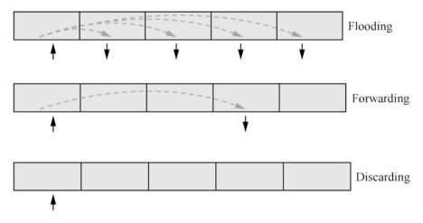
Fig. 4.12 Actions by the switch on frames
