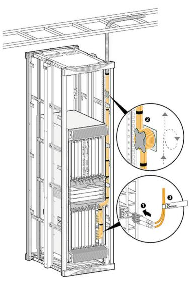
Fig. 3.55 Connect the optical fibers
