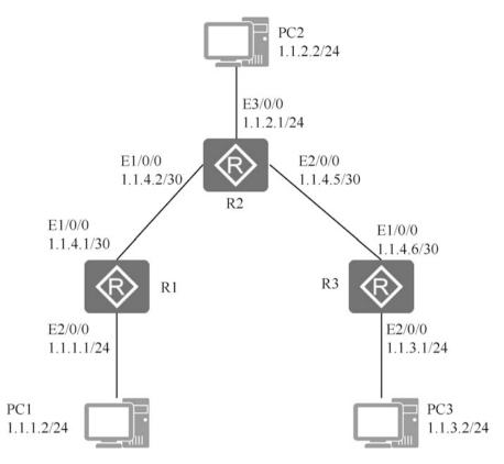
Fig. 5.24 Topology of static routing configuration
