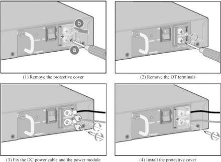
(3) Fix the DC power cable and the power module
