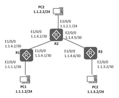
Fig. 4.29 Network topology of static routing
