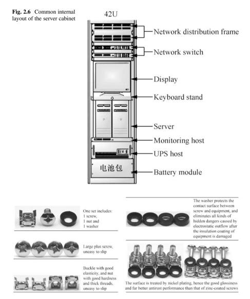
Fig. 2.7  $M6 \times 16$  screws for cabinet
