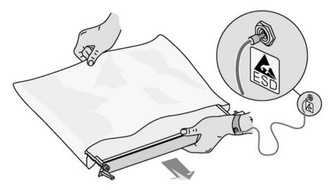
Fig. 1.2 How to wear an ESD wrist strap
