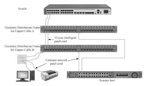
Fig. 2.10 Systematic connection of the twisted-pair distribution frame
