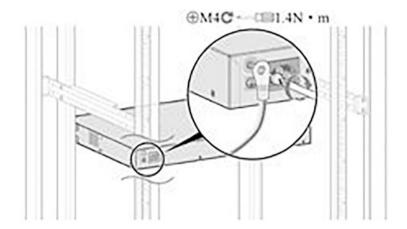
Fig. 3.62 Connect the grounding cable to the switch grounding point
