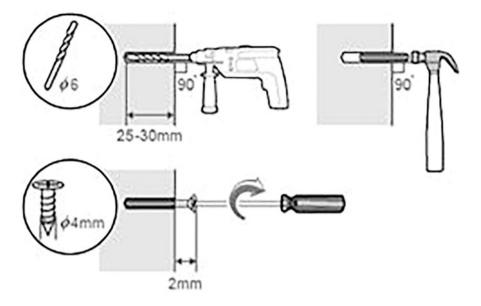
Fig. 3.110 Drill holes and mount the screws
