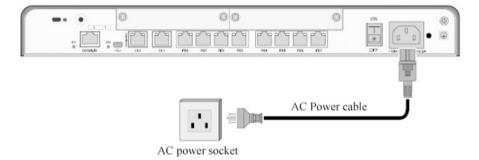
Fig. 3.34 Connect the power adapter
