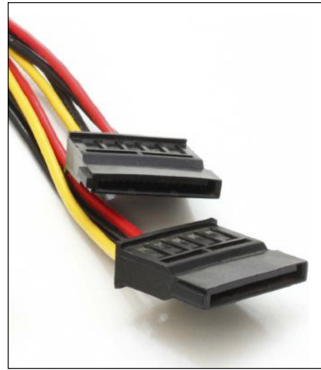
Figure 2.8 A power connector for a Serial ATA (SATA) hard drive. The drive requires both +5 and +12 power, supplied on the red and yellow wires, respectively.
