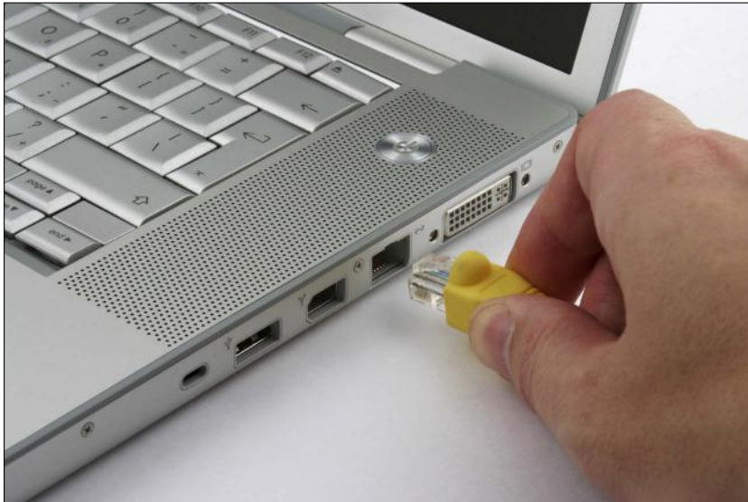
Figure 1.14 Ethernet is the most common type of network connection. Most computers have an Ethernet port.
