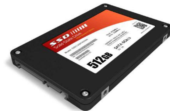
Figure 3.30 A solid-state hard drive looks much like an HDD from the outside.
