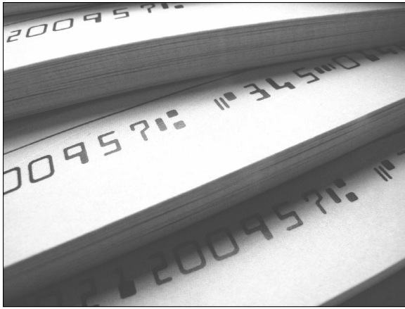
Figure 3.12 The routing numbers on checks are written with magnetic ink so they can be read by MICR machines.
