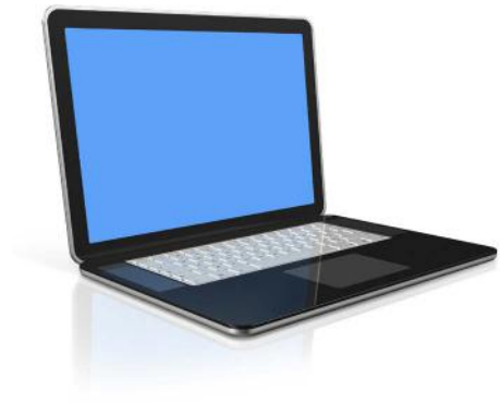
Figure 1.3 A notebook PC has a built-in monitor, keyboard, and pointing device, such as a touchpad.
