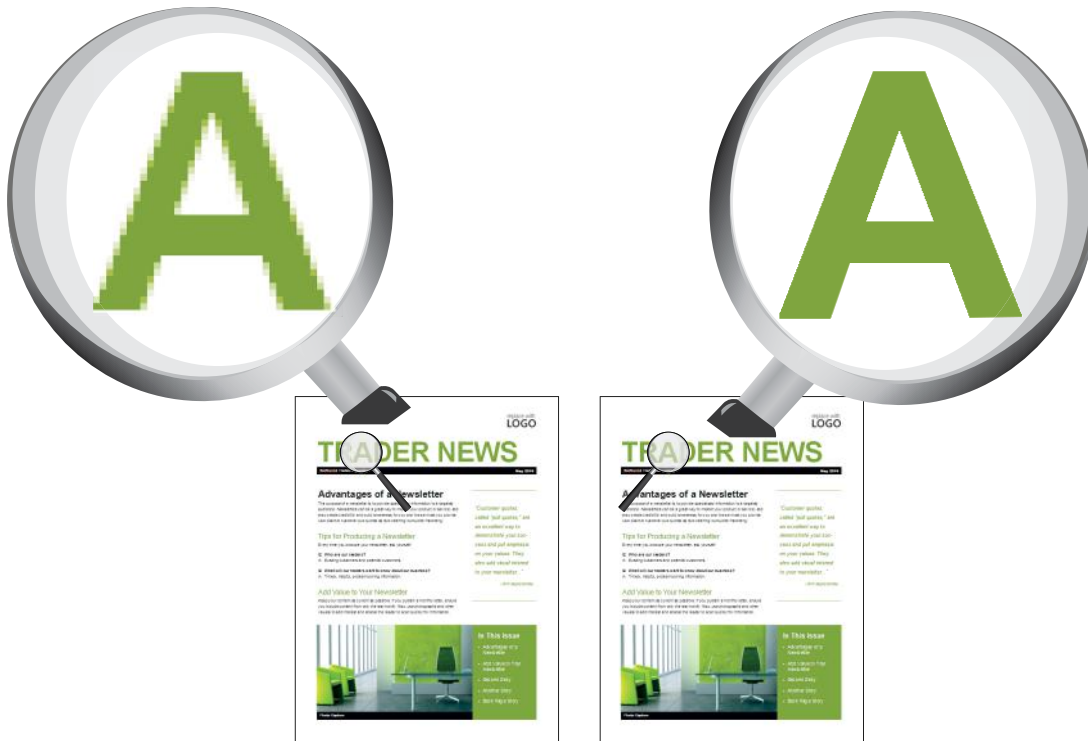
Figure 3.21 A high-resolution printout uses more pixels per inch, resulting in smoother lines and finer details.
