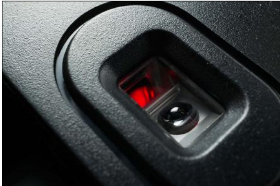
Figure 3.3 The underside of an optical mouse contains a red light and a sensor that measures its reflection from the surface the mouse is used on.
