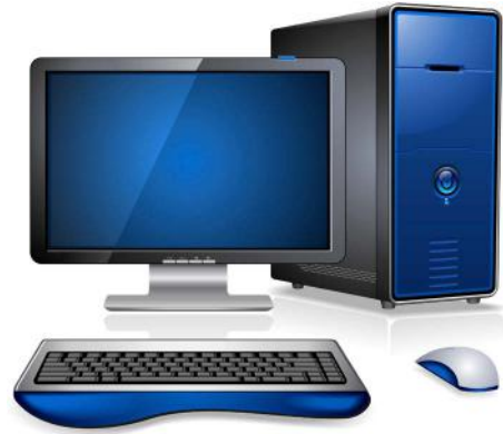
Figure 1.2 A desktop PC contains a separate system unit, monitor, keyboard, and mouse.
