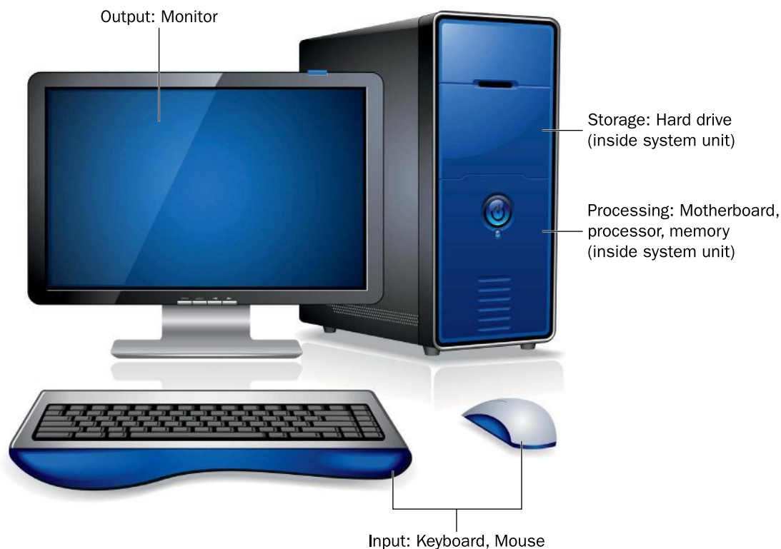
Figure 1.11 Components of a typical desktop computer system.
