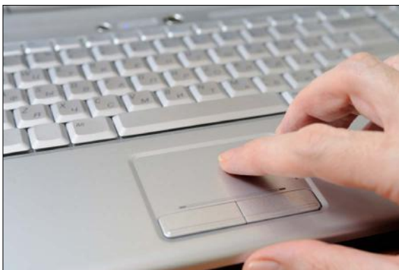
Figure 3.5 A touchpad is a touch-sensitive area that the user drags a finger across to move the pointer onscreen.
