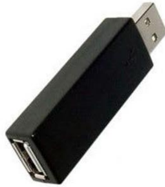
Figure 11.2 A hardware keylogger. This model looks similar to a flash drive.
